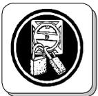
Prior to any repair works on the machine and its drives, secure the machine against unintentional switching-on. Pull out the mains plug in order to do this.
